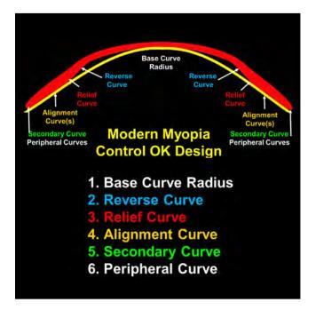
Figure 6a: Designs with five to six curves or zones and small optic zones may lead to even better overall fitting of OrthoK and expanded use in eye care practices around the globe.
