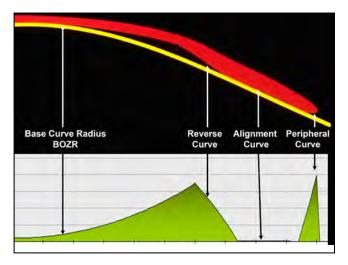
Figure 5: The construction of OrthoK designs continued to morph as innovators with four to five curves (or zones) attempted to improve fitting characteristics.
