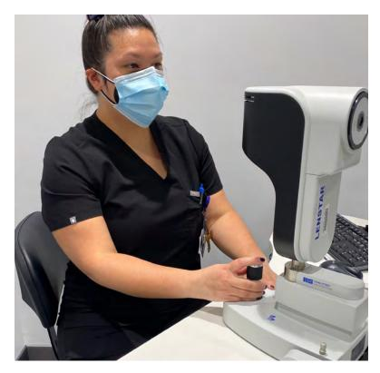
Myopia progression is best assessed by axial length measurements using an optical biometer.
