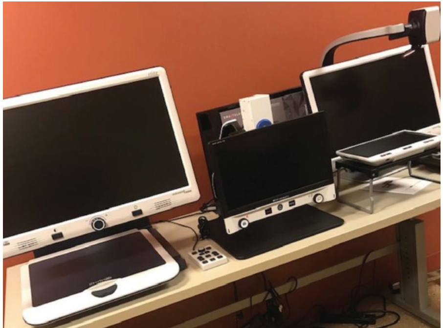
Fig. 3. Left to right: Distance-enhancement interfaces corresponding to the aforementioned binocular telescope, monocular telescope and Max TV glasses of Fig. 2, respectively.
