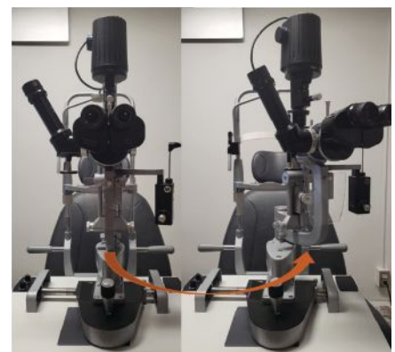
Fig. 2. The entire ocular-light source unit can be turned to adjust the orientation of the light source.
