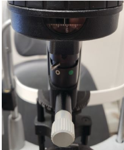
Fig. 4. Use the calipers on your slit lamp beam to measure.
