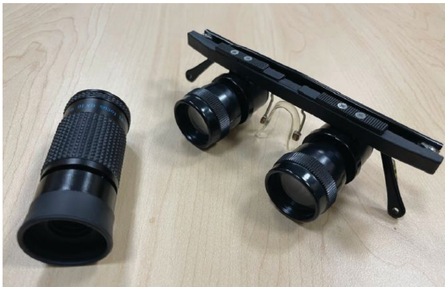
Fig. 3. A monocular handheld telescope (left) and a binocular telescope in a frame.
