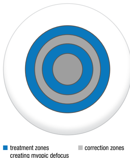
Fig. 2. The MiSight lens has two treatment zones, creating a peripheral myopic defocus that causes the image to focus in front of the retina and slow axial elongation. Myopia is corrected in all gaze positions. Image: adapted from CooperVision.
