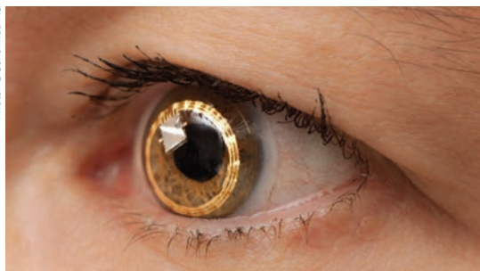
Fig. 2. The Triggerfish contact lens sensor monitors IOP over a 24-hour period.
