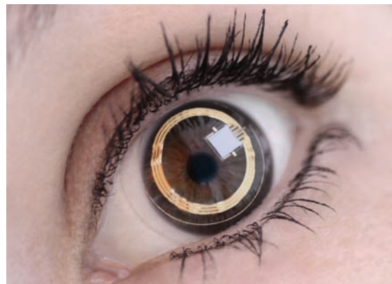
Sensimed’s Triggerfish lens records changes in corneal curvature that correspond with intraocular pressure.
